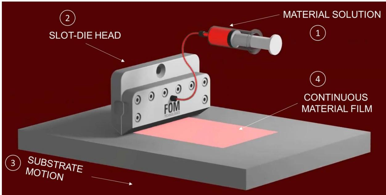
Slot-Die Coating is a highly scalable technique for depositing thin and uniform material films with minimal waste and low operational cost. It was invented in the 1950's by Eastman Kodak Co. for the production of photographic films. Since then, it has seen widespread adoption in industrial manufacturing of electronics, packaging and pharmaceuticals.
