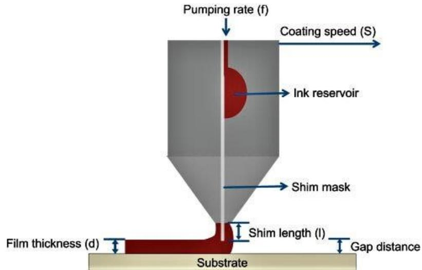
A key benefit of Slot-Die Coating is its “pre-metered” nature. This means that the coated wet film thickness ( $d$ ) can be easily controlled and calculated from the pump rate ( $f$ ; the rate at which ink enters the system), the substrate motion speed ( $S$ ; the rate at which the substrate accepts ink from the system), and the coating width ( $W$ ; the width across which the ink is dispersed upon the substrate).<sup>4</sup>
